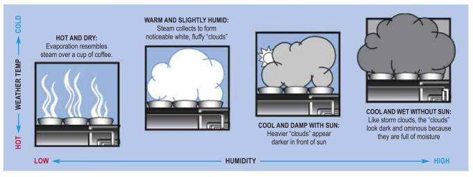
This illustration depicts the look of the "clouds" coming out of the top of the cooling tower stacks based on the atmospheric conditions on a given day. Beyond the temperature and humidity of the surrounding air, the appearance of the "clouds" is also affected by the angle of the sun: if it is behind the "clouds" they appear darker. The wind also affects the appearance: on windy days steam mixes with the surrounding air more quickly.
